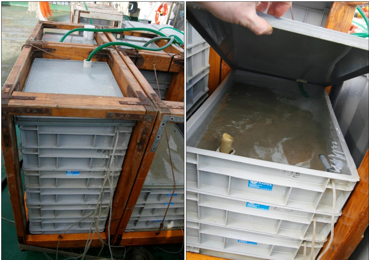
Figure 5 – Holding facilities were supplied with a continuous flow of sea water. Two individuals were accommodated in each of the tank: 1 plaice and 1 sole, enabling easy identification of the individuals.
