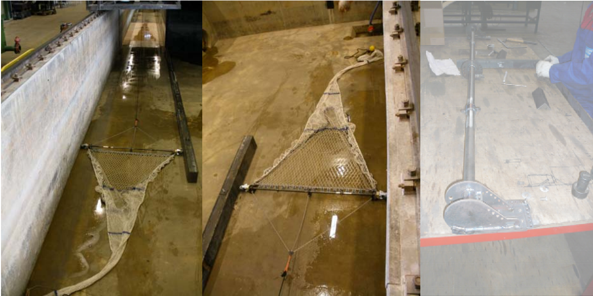
Figuur 3-3: Model 1:6 in de water-grond goot van DELTARES
