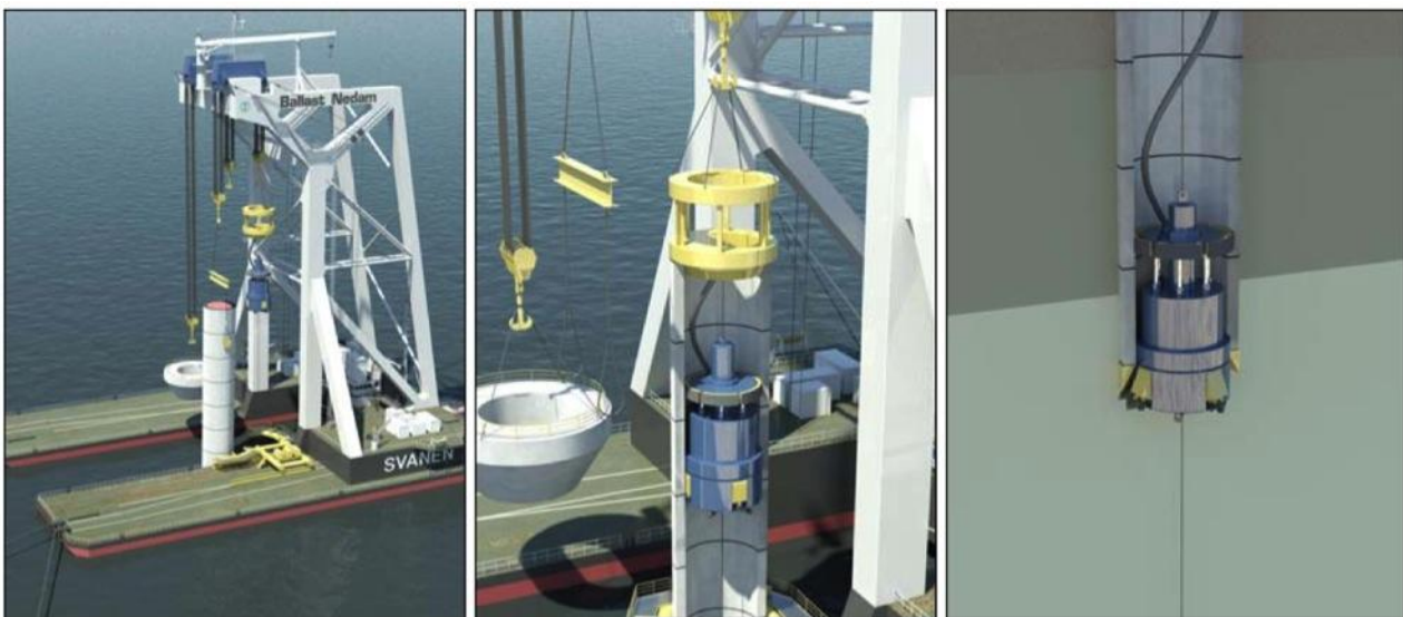
Figure 42. Drilled concrete monopile concept by Ballast Nedam (van der Meer & van Bergen, 2009)
