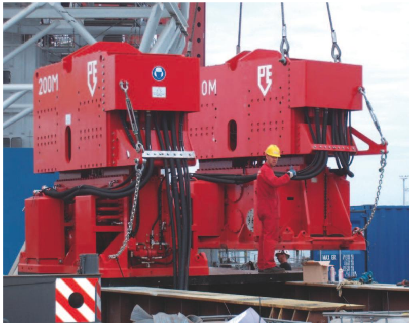
Figure 38. Two PVE 200 M vibratory hammers joined together (Dieseko Groep B.V., 2009)
