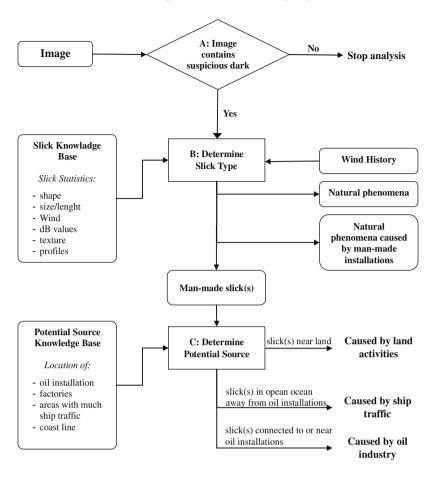
Fig. 1. Flow diagram for the detection of slicks in SAR images, Furevik et al. (2005).
