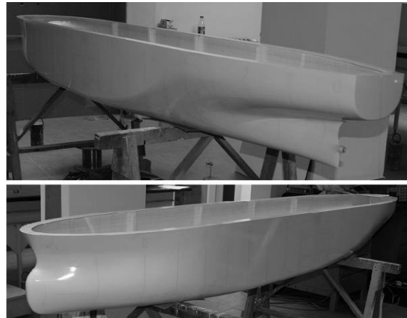
Figure 6 Stern and stem section of the SS model in fibre glass reinforced vinyl ester.
