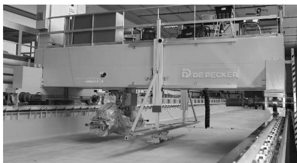
Figure 2 Shallow water towing tank (empty) at Flanders Hydraulics Research with secondary beam
