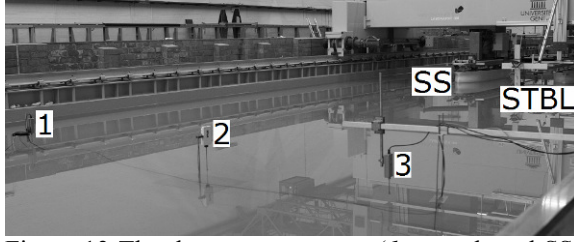
Figure 13 The three wave gauges (1 at starboard SS, 2 between ships and 3 at port side STBL)
