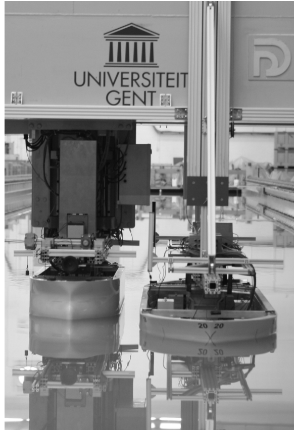
Figure 7 Ship-to-ship interaction tests
