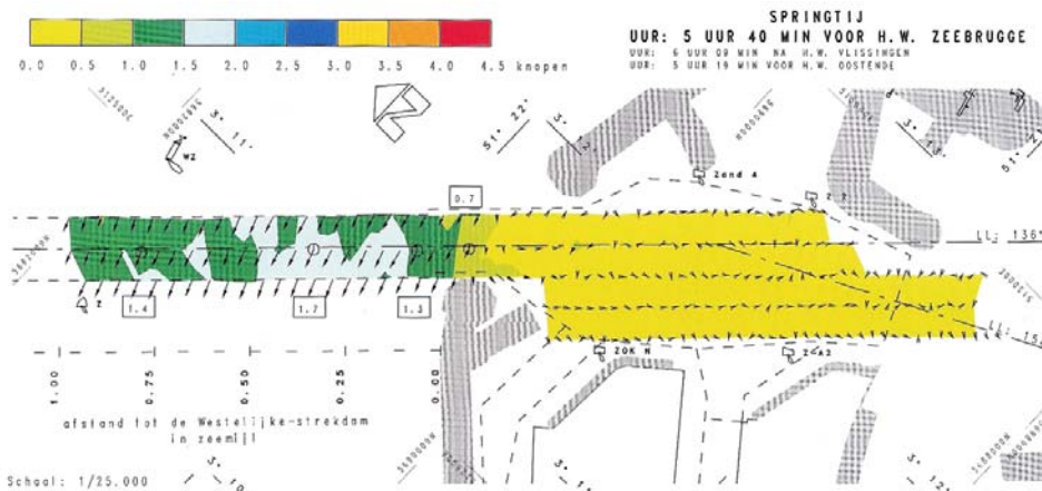
Figure 7.30. Current in the access channel of the harbour of Zeebrugge, 5h40min before spring-tide [7.3].
