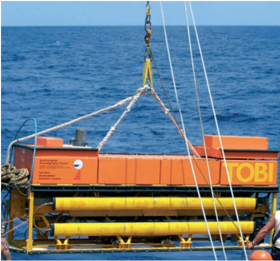
Photo 3.10: TOBI (Towed Ocean Bottom Instrument) is one of the UK deep sidescan sonars used to produce acoustic maps of the deep seafloor
