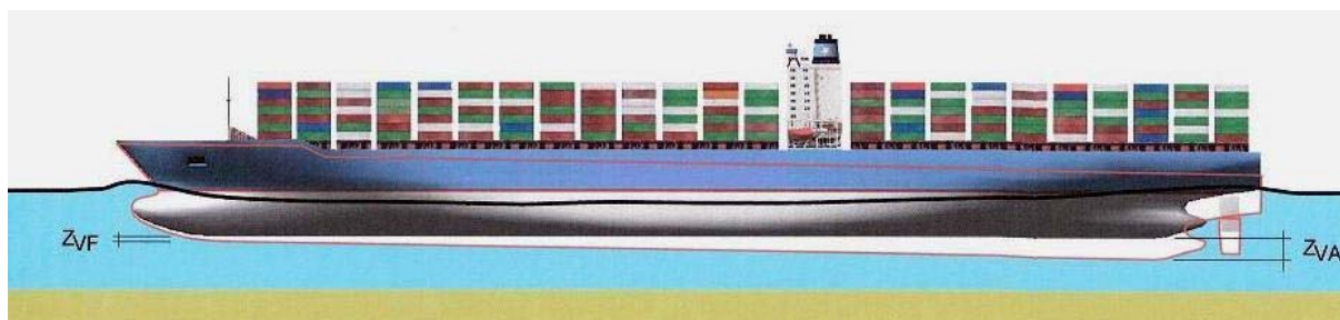
Fig.2 Definition of ship squat as combination of sinkage and trim
