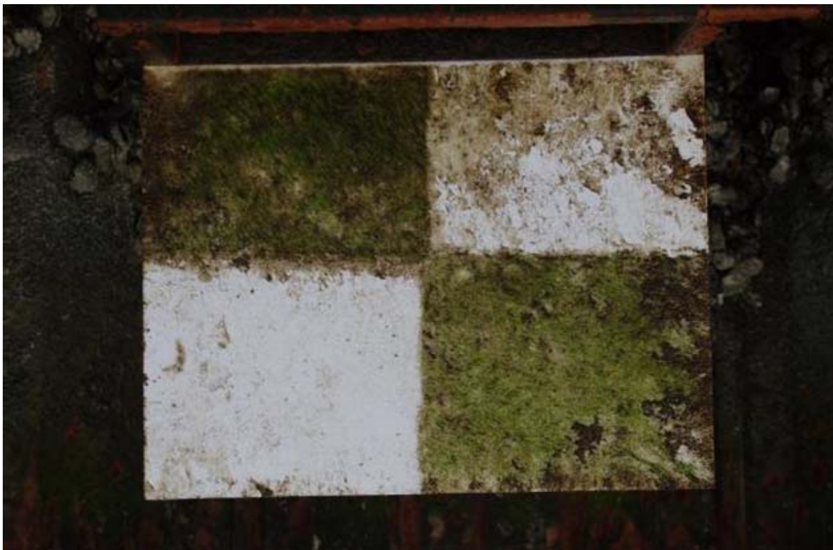
Left test plate. Top left and bottom right: Control paint coated. Top right and bottom left: Intersleek 1100SR coated.
