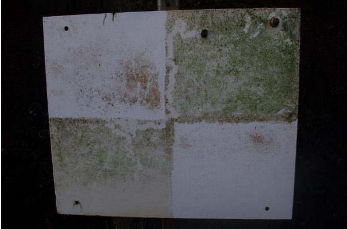
Control plate. Top left and bottom right: intersleek 1100SR coated. Top right and bottom left: Control paint coated.
