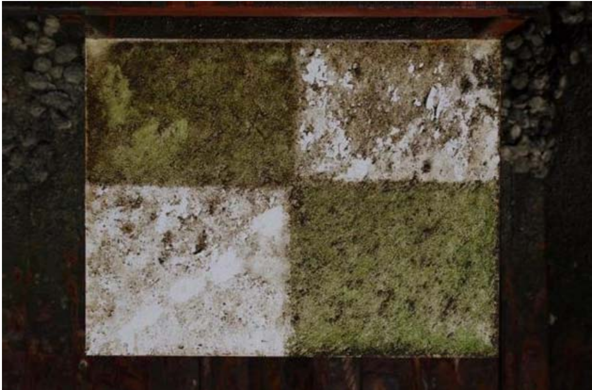
Right test plate. Top left and bottom right: Control paint coated. Top right and bottom left: Intersleek 1100SR coated.
